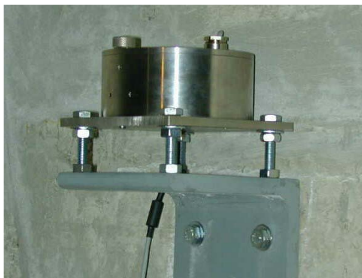
Figure 3: Inclinometer in its case allowing a full 180° rotation to compensate for drift
