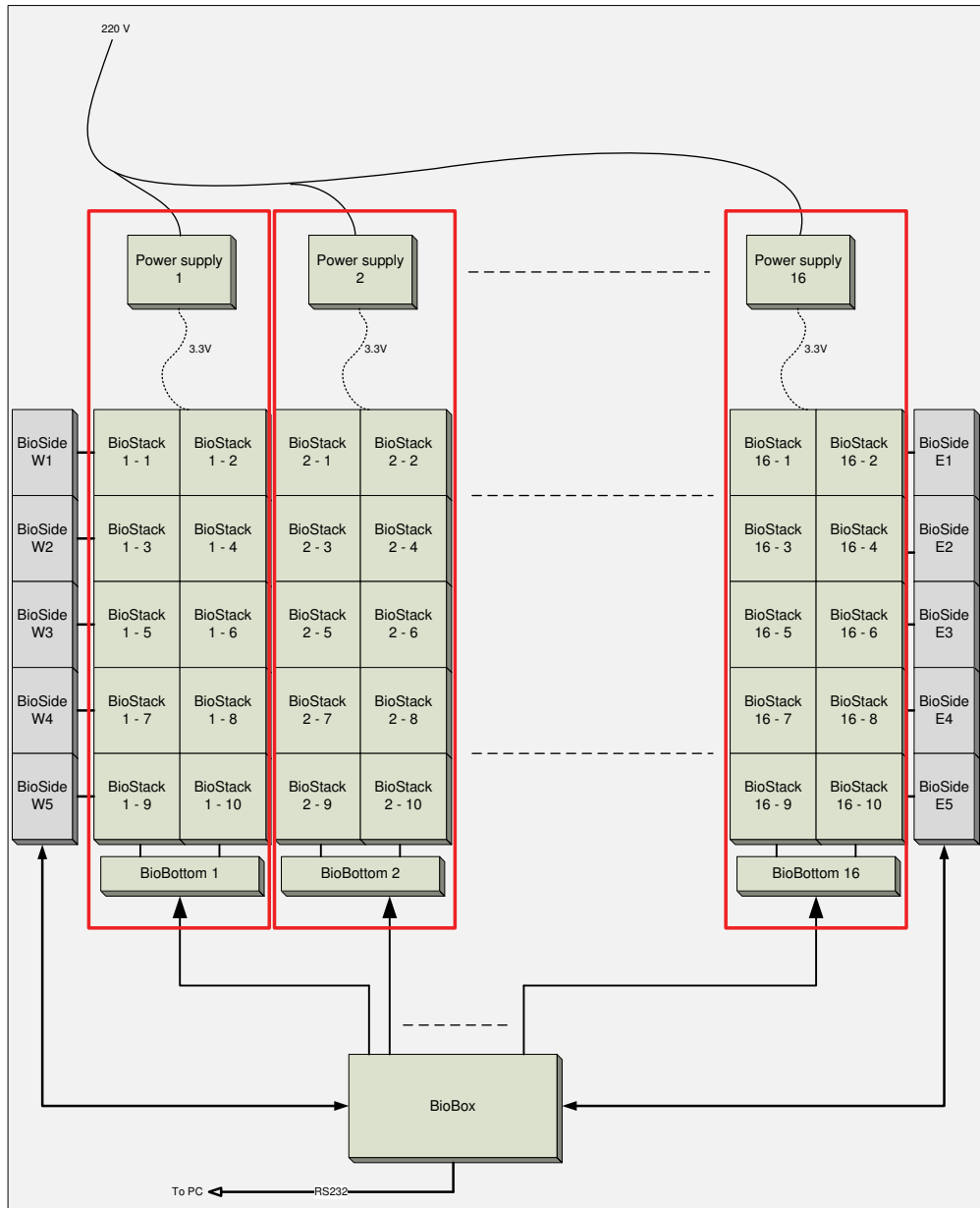
Figure 3.10: Schematic of the BioWall architecture; each red rectangle correspond to a rack.
