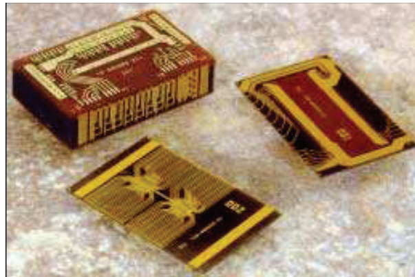
Figure 2.9: Two individual ICs at the bottom-right and a stacked chip made of 19 layers of these ICs. Source: [58]
