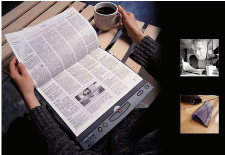
Figure 9.2: Electronic newspaper; control case at the bottom with its flexible display. Source: IBM.
