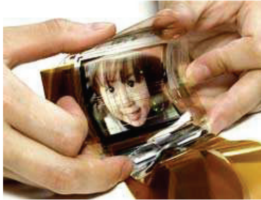
Figure 9.4: Color screen, thin and bendable like a paper sheet. Source: Sony ® .
