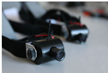
Fig. 1. The WearCam, a 42 grams head-mounted wireless camera.
