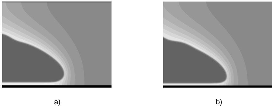
Figure 5-5 Stationary dendrite tip shapes growing at 530°C. a) \alpha=5^\circ , b) \alpha=15^\circ . For the case with \alpha=15^\circ , the apex of the tip is closer to the boundary, the gap of solute-rich liquid between the solid and the boundary is thinner and the minimum curvature is smaller.
