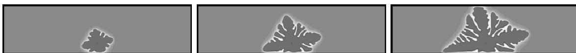
Figure 4-33 Simulation of a dendrite nucleated in the bulk and approaching the boundary. The dendrite tip does not establish contact with the boundary regardless of the imposed wetting condition. All other simulation conditions are the same as in Figure 4-31 except the positioning of the nucleus.
