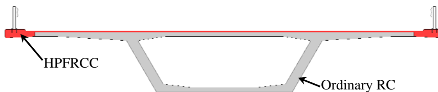
Fig. 1. Conceptual vision of a hybrid bridge deck with a protective layer of HPFRCC.
