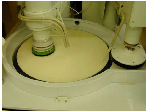
Fig. 3.2: Photo of the main CMP setup used in this work (polishing head on the left, conditioning head on the right, polishing pad at the bottom).
