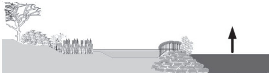
Figure 3.6: Possible method for enhanced transitional zone in a heavily fluctuating reservoir. During low flow the transitional zone remains submerged. Culvert filling takes place during high flows
