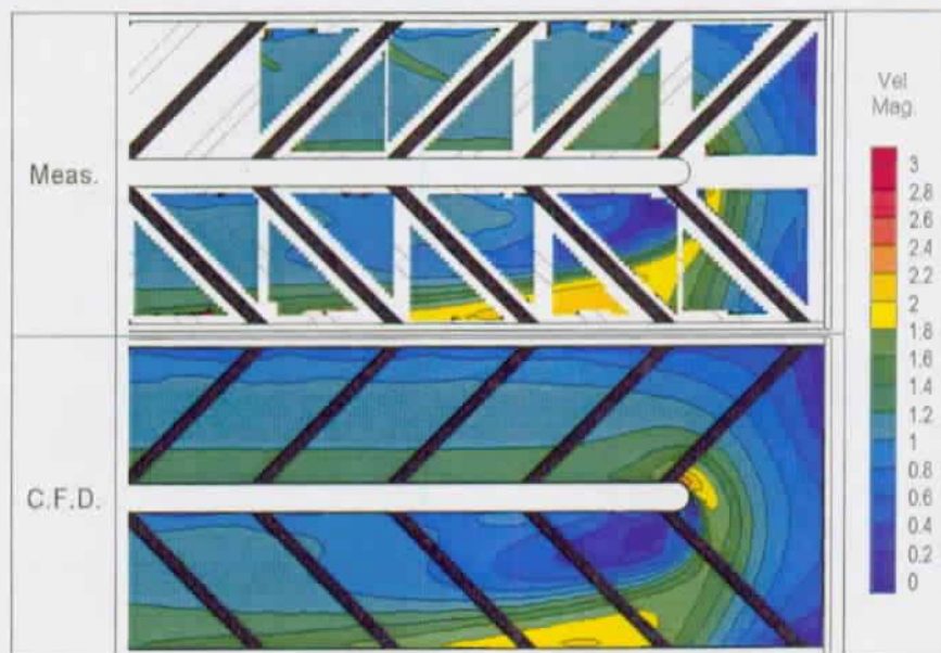
Figure 82: CFD prediction of the baseline configuration centre plane velocity magnitude (baseline configuration, Re=50,000 ).
