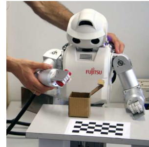
Fig. 1. A human operator kinesthetically demonstrates a task to the robot, i.e. by grabbing and moving its limbs while the robot records joint angle trajectories.
