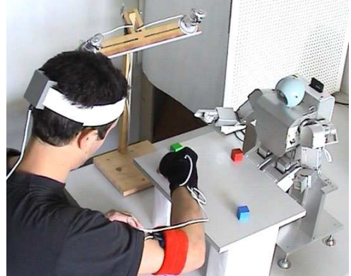
Fig. 1. Experimental setup. The user is pointing at an object while the robot is observing his gesture using motion sensors.
