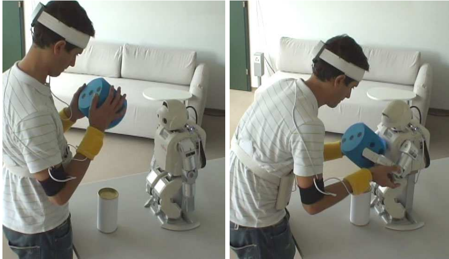
Figure 1. Different modalities are used to convey the demonstrations and scaffolds required by the robot to learn a skill. The user first demonstrates the whole movement using motion sensors ( left ) and then helps the robot refine its skill by kinesthetic teaching ( right ), that is, by embodying the robot and putting it through the motion.
