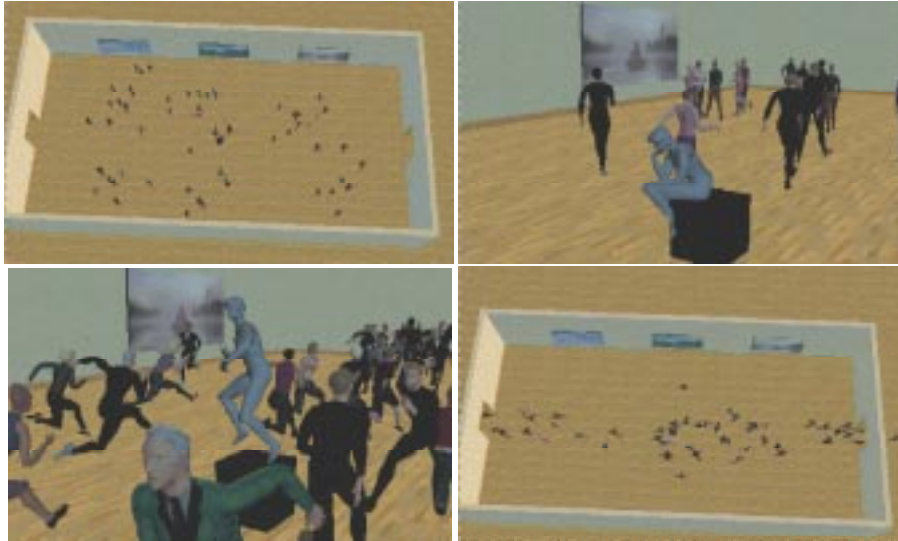
Figure 5: Scenes of simulation of evacuation due to a panic situation. Up left and right: Before the event, the crowd walks. Down, left and right: crowd reacts. The statue motion and action are externally controlled.
