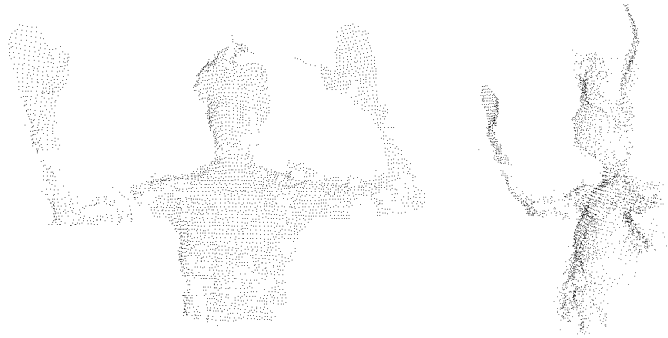
Figure 5. 3-D point cloud after passing filtering
