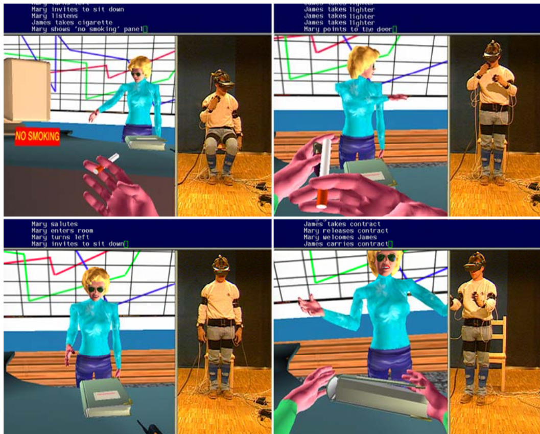
Figure 4. A virtual office environment with the participant (right), his avatar (virtual camera view) and a digital character (cyan). The animation automata is driven by the recognition events of the performers actions.
