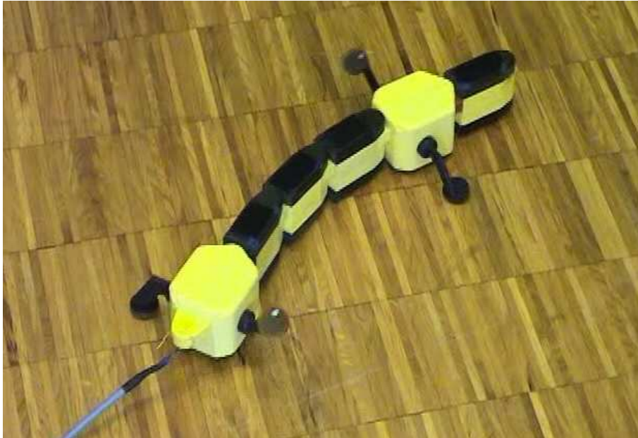
Figure 3.5: The prototype of salamander robot built with the first generation elements.
