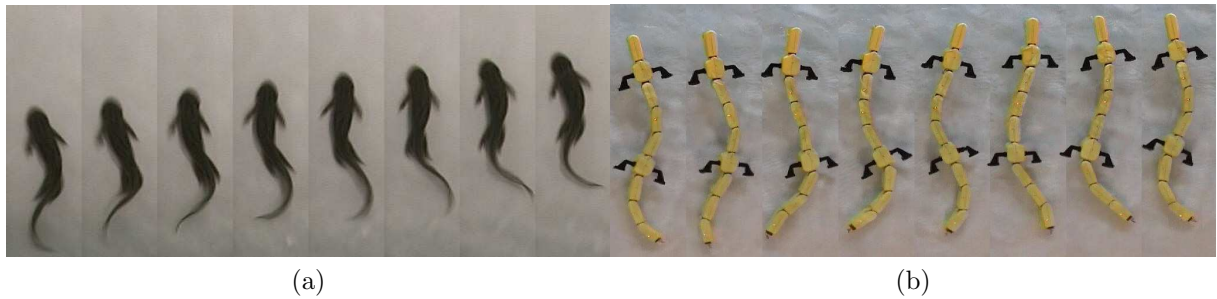
Figure 6.8: Snapshots from videos for salamander (a) and robot (b) swimming. The time step between the snapshots is 0.04 s for the salamander, and 0.12 s for the robot.
