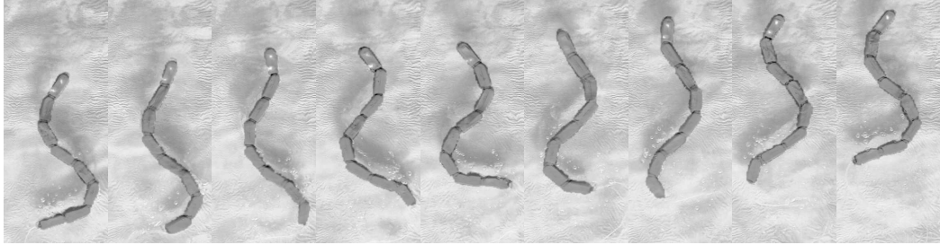
Figure 7.5: The robot swimming at A = 53^\circ , N \cdot \Delta\phi = 1.05 , \nu = 1.0 Hz and \alpha_1 = 0.82 . The time step between the snapshots is 0.12 s. Videos of the robot are available at http://birg.epfl.ch/amphibot .
