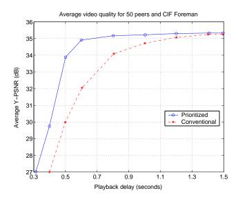
Figure 3. Average Y-PSNR (dB) vs. Playback delay for CIF Foreman and 50 peers.
