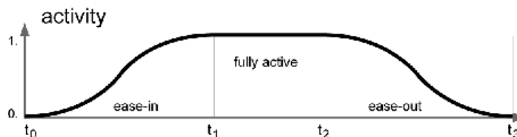
Figure 4: Default activity profile with cubic steps for ease-in and ease-out. The key times can be arbitrarily set over the original motion duration [t_1, t_F] .
