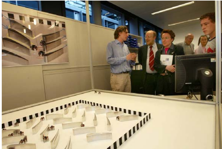
Figure 3. A simple 2D mock-up of a turbines interior, which allows us for modeling and designing swarm coordination, independently from the upside-down locomotion problem. Image © Alain Herzog.
