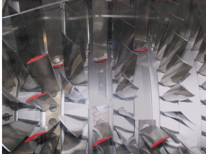
Figure 2. A close-up on the compressor section of a medium-size jet turbine engine. The distance between blades is approximately four centimeters.
