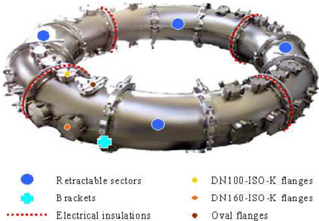
Figure 2.2: The TORPEX vacuum vessel, composed of twelve sectors, four of which are 'retractable'. Several of the 48 ports are visible.
