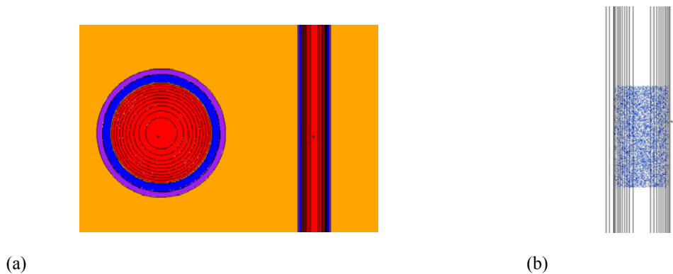
Fig. 3.4: Fuel pin in MCNP model of the NEUTRA setup: on the left (a) the internal composition described using different colours (fuel matrix, cladding and over-cladding) and on the right (b) the simulated vertical source distribution.
