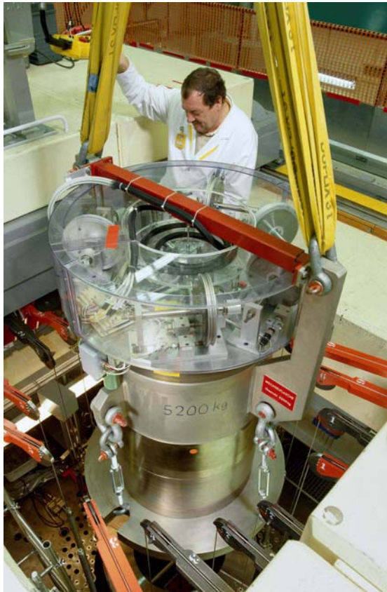
Fig. 3.2: PROTEUS transport flask/sample changer used for preliminary measurements of spent fuel rod segments.
