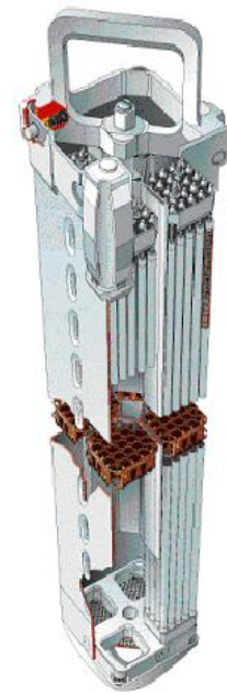
Fig. 1.1: SVEA-96 fuel assembly (BWR).
