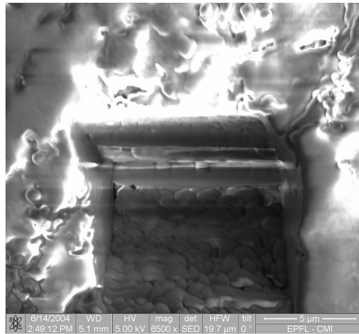
Figure 2.11: Charging of a cement sample in Focussed Ion Beam
