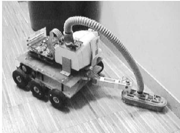
Figure 4: Koala robot modified and equipped with an arm.
