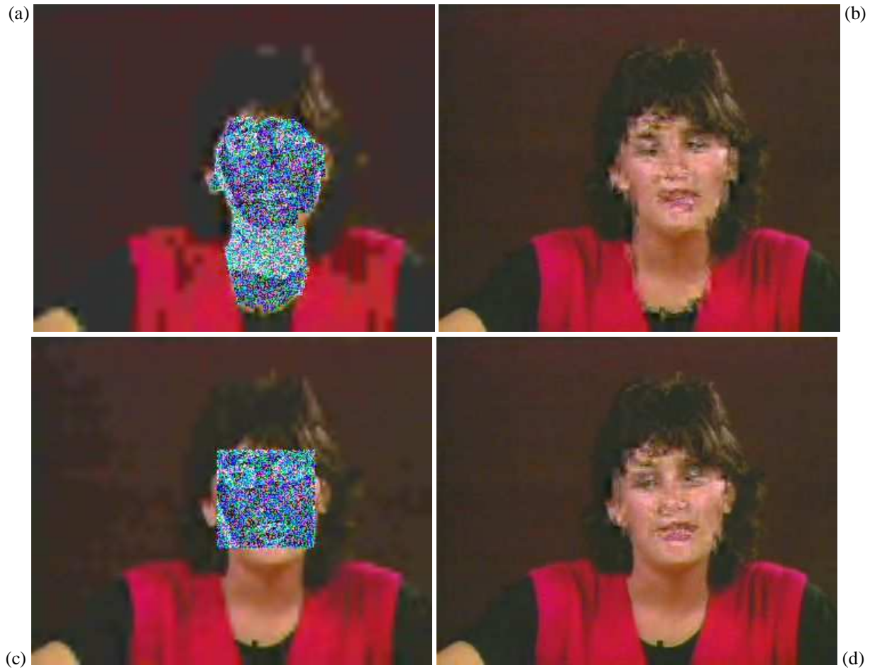
Figure 9 – Image-domain versus transform-domain scrambling for Motion JPEG 2000 at 2 Mb/s (a) skin detection mask and image-domain scrambling (b) skin detection mask and transform-domain scrambling (c) face detection mask and image-domain scrambling (d) face detection mask and transform-domain scrambling.
