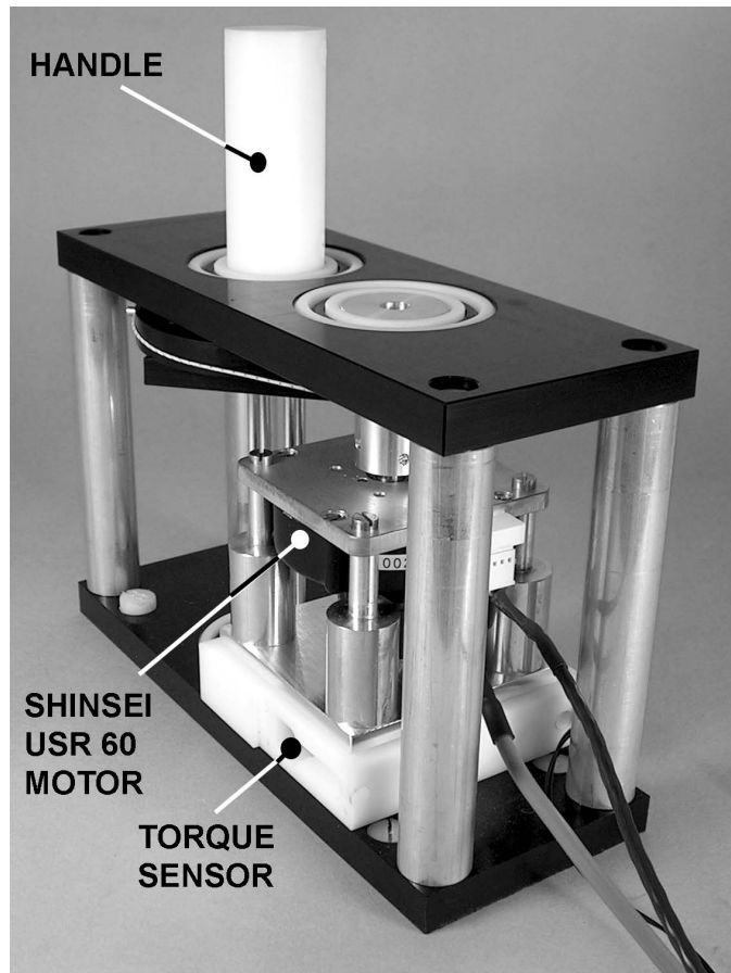
Fig. 2. Prototype of the MR compatible 1 DOF haptic interface.
