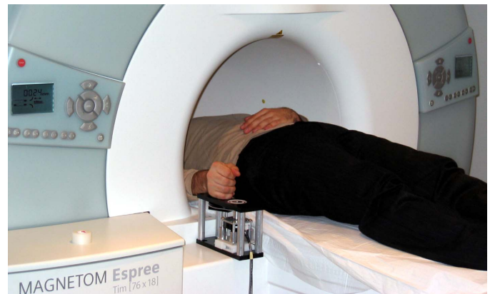
Fig. 1. Testing of the haptic interface prototype inside an MR scanner at the University Hospital in Basel.
