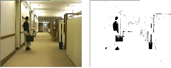
Figure 2: Example of shadow selection map. (a) Frame 37 of the test sequence Hall Monitor and (b) corresponding shadow selection map. The black labels identify pixels that are not considered in the colour analysis stage
