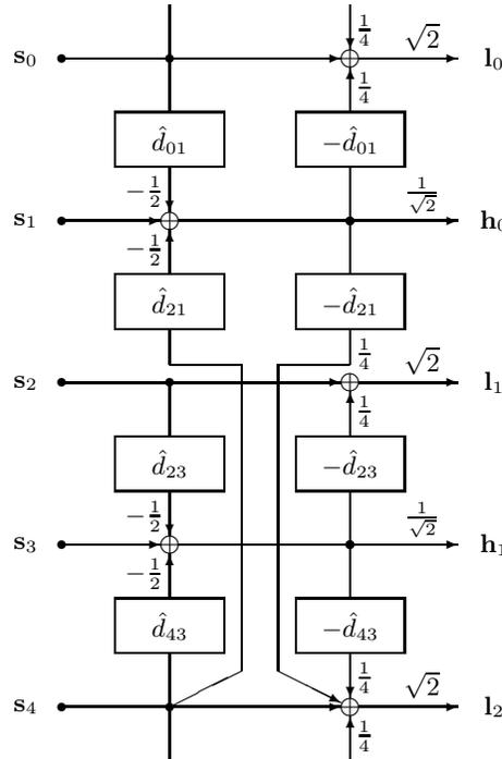
**Fig. 6.** Example of the first decomposition level of the 5/3 transform with frame-adaptive motion-compensated lifting steps. The frames  $s_0$  and  $s_4$  are used to predict frame  $s_1$ .
