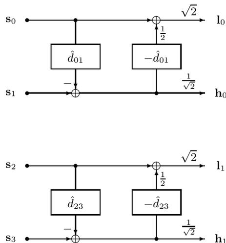
**Fig. 1.** First decomposition level of the Haar transform with motion-compensated lifting steps. A fix reference frame structure is used.
