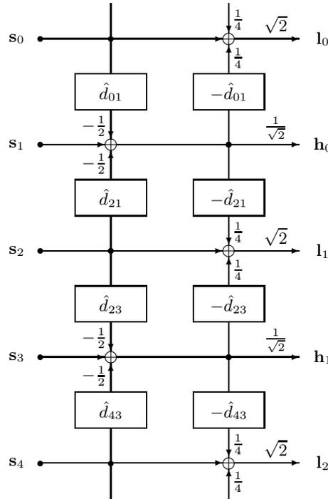
**Fig. 5.** First decomposition level of the 5/3 transform with motion-compensated lifting steps. A fix reference frame structure is used.
