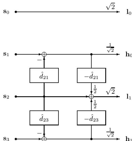
**Fig. 2.** Example of the first decomposition level of the Haar transform with frame-adaptive motion-compensated lifting steps. The frame  $\mathbf{s}_2$  is used to predict frame  $\mathbf{s}_1$ .
