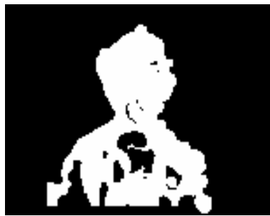
(c) Moving area mask performed over a median filtered (5x5) version of the module(thresholded at 0.04).
