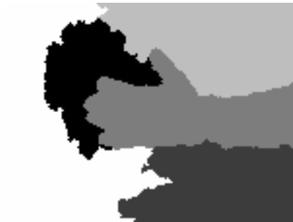
(a) Segmentation of the image Rosa's hand, using the three components with weights W_{\mathcal{C}_i} = 1.0 , W_{\mathcal{C}_m} = 0.4 , W_{\mathcal{C}_g} = 0.4 and filtered with the morphological filter. Level of segmentation: \sigma_n = 50 pixels
