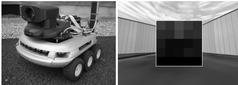
Fig. 1. Left: The original six-wheeled robot Koala equipped with a pan/tilt camera. Right: The robot's perspective in a simulated environment. The robot can access the world with 5 by 5 retina at the center of the image.
