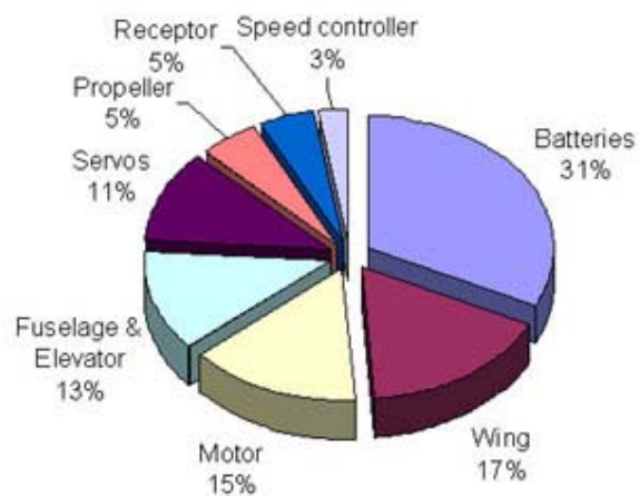
Figure 13. Weight distribution of our prototype indoor slow flyer, the model C4. 100% corresponds to 45 g.
