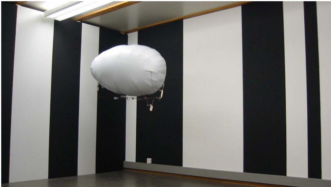
Figure 9. The evolutionary blimp in its environment, a 5 by 5 meters room with randomly spaced stripes on walls.
