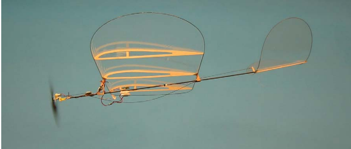
Figure 11. A prototype of the indoor autonomous flyer with bi-directional digital communication using Bluetooth. Main features: weight of 45 g, 82 cm wingspan, 1.4 m/s minimum flight speed, and vectored thrust for steering (the motor-gear-propeller system is articulated about the yaw axis).
