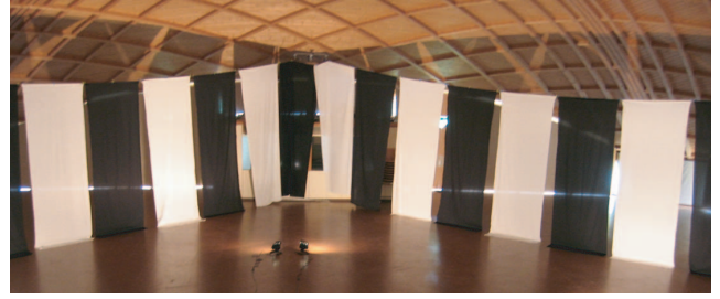
Fig. 6. Part of the square arena (16 by 16 meters) used for obstacle avoidance experiments with the flying robot. The walls are made of black and white curtains. Note that the regularity of the pattern is due to the default material size.
