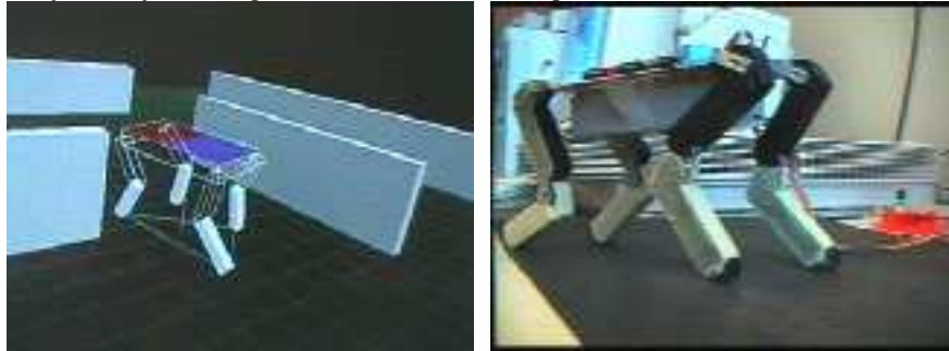
Fig. 9. An evolved 4 legged robot. The control system of the robot, its body size, and length of legs have been evolved in 3D simulations (left). The physical robot (right) has been built according to the evolved genetic specifications. The evolved control system is transferred from the simulated to the physical robot. Such evolved robot can walk and avoid obstacles. The robot is approximately 20 cm long and less than 1kg without batteries. Leg control performed by a set of HC11 microcontrollers.
