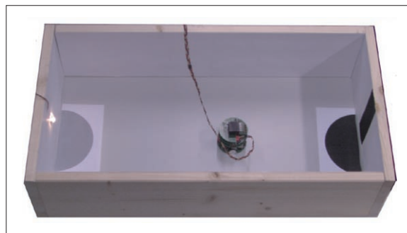
Fig. 4. A mobile Khepera robot equipped with a vision module can gain fitness points by staying on the grey area under the light bulb only when the light is on. The light is normally off, but it can be switched on if the robot passes over the black area positioned on the other side of the arena. The robot can detect ambient light and wall colour, but not the colour of the floor.
