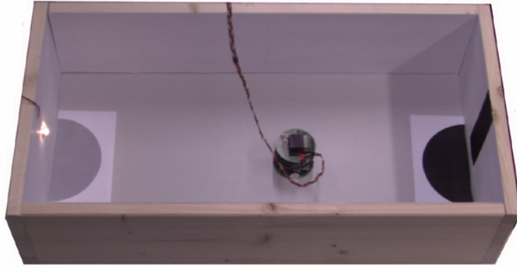
Fig. 1. A mobile robot equipped with a vision module gains fitness by staying on the gray area only when the light is on. The light is normally off, but it can be switched on if the robot passes over the black area positioned on the other side of the arena. The robot can detect ambient light and the color of the wall, but not the color of the floor.
