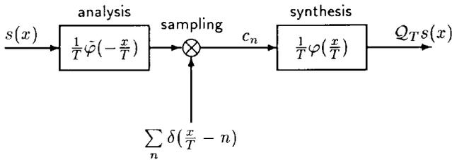
Fig. 1. Block diagram representation of the approximation operator  $\mathcal{Q}_T$ . The boxes represent continuous-time filters characterized by their impulse response. Sampling is modeled by a multiplication with a train of Dirac functions. When  $\tilde{\varphi}(x) = \delta(x)$  (identity operator), the system is an interpolator. The operator is a projector if and only if  $\varphi$  and  $\tilde{\varphi}$  are biorthonormal.
