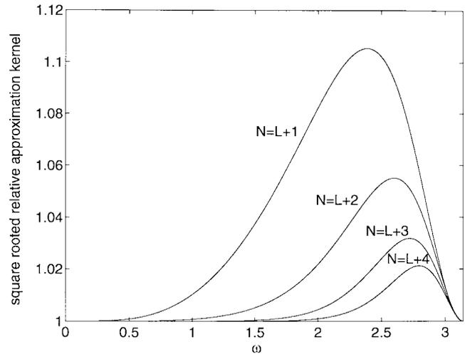
Fig. 6. Optimal cubic spline ( $L = 4$ ) quasi-interpolants: reduction of the error as the order  $N$  of the windowing B-spline increases (the same convention as in Fig. 5 has been used for the plots of the kernels).
