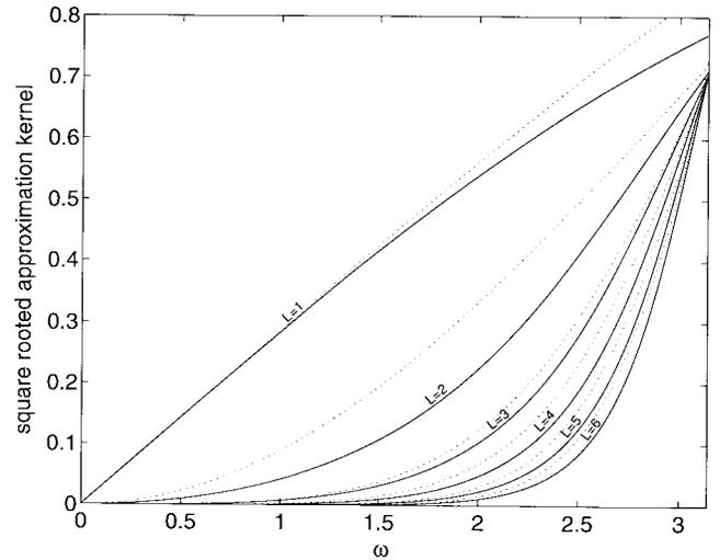
Fig. 3. Least-squares (solid lines) and interpolating (dotted lines) rooted approximation kernels for the B-splines of order 1 to 6. The kernel is all the closer to the  $\omega$ -axis as the approximation order is higher.
