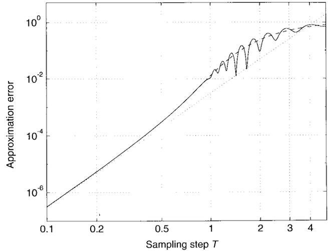
Fig. 2. Least-squares approximation error of the function  $s(x) = e^{-\frac{x^2}{2}}$  by cubic splines as a function of the sampling step  $T$ . The error estimate  $\eta_s$  (dashed line) is an unbiased smoothed version of the true error (solid line), as stated in Theorem 2; the dotted line is the first order asymptote  $C_\varphi^- \|s\|_{\mathbf{L}^2} T^4$ , computed according to [21].
