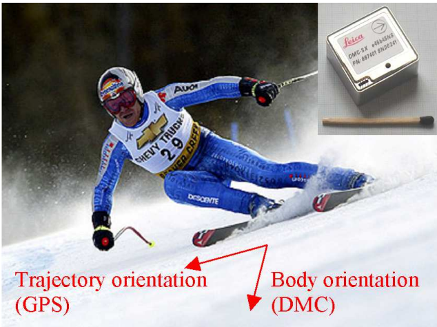
Figure 6: The DMC (inset) and the GPS antenna are both mounted on skier's helmet. The azimuth derived by the former is related to direction of movement while the one of DMC/GPS is associated with the orientation of skier's body.
