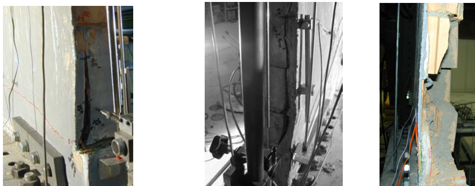
Figure 4.11: Development of vertical cracks between retrofitting material and masonry panel
