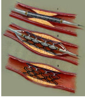
Figure 4: Balloon expandable stent. (1) Stenosis in a artery; the internal balloon is inflated and it plastically deforms the stent. (2) The stent constitutes a real scaffolding for the artery that recovers again the original lumen. (3) The balloon is deflated and then pulled out, while the stent is left inside the artery.
