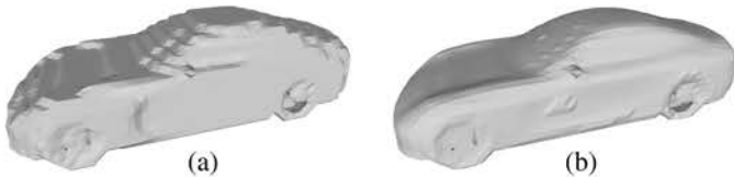
Fig. 14. Marching Cubes on an occupancy field. (a) running Marching Cubes on the occupancy field predicted by f_{\Theta} yields artifacts. (b) Using an inverse sigmoid function to amplify the predicted occupancy values yields smoother shapes.
