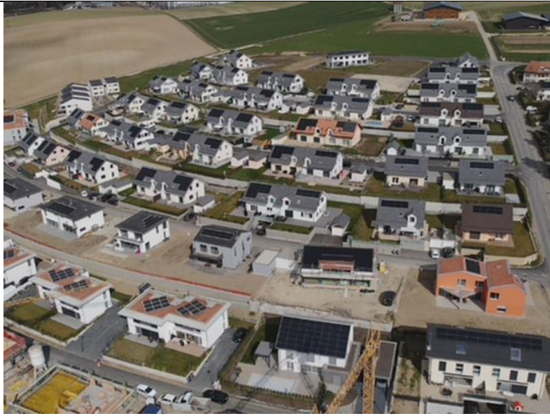
Figure 8 – Against minimal requirements. Aerial view of a newly built residential housing project recently realized in Bussigny (Switzerland). In this specific case, only 10 m 2 of solar PV was installed on most single-family houses – being fully compliant with the local building requirements - when in reality 100+ m 2 (of well oriented PV) could have been installed on most roofs (credits: Thomas Söderström).
