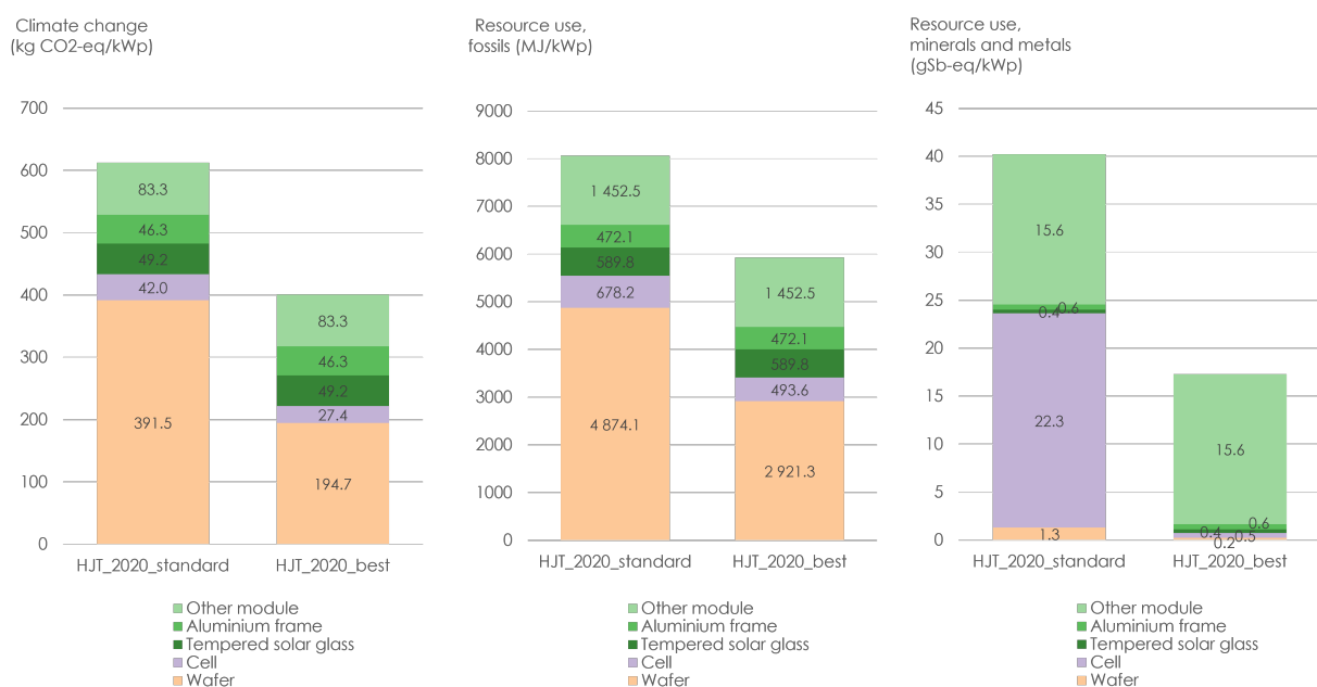
Figure 4.2: Environmental footprint per kWp of HJT technology (standard vs best practice) for CC, RUF and RUM impact categories. EF 3.0 impact assessment methodology used. Activities included : wafer production and transport, Cell and Module manufacturing in Europe, end-of-life modeled separately. Activities excluded: BOS & Installation manufacturing, use phase. Chinese electricity mix: 1023 g CO 2 -eq/kWh ; European electricity mix: 418 g CO 2 -eq. Standard: China 2020 wafer (170 \mu m), sc-Si bifacial HJT cell, Ag paste for metallization (220 mg/ M6 wafer), ITO for TCO, module efficiency \eta=21.75\% . Best practice: Norsun wafer (170 \mu m), sc-Si IBC HJT cell, copper plating for metallization, AZO for TCO, module efficiency \eta=21.75\% . All other parameters are identical to standard.
