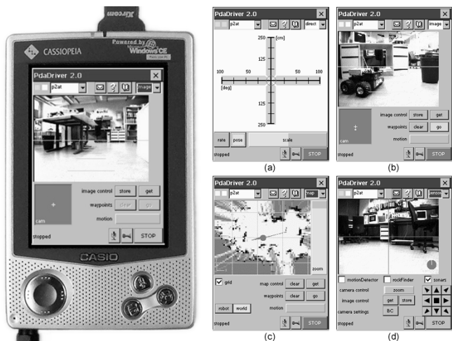
Fig. 1. PdaDriver and control modes. (a) Rate/Position. (b) Image waypoint. (c) Map waypoint. (d) Sensor.
