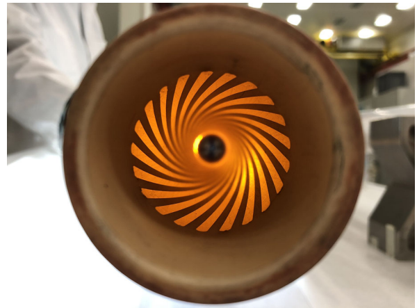
FIG. 18. Photograph of the prototype helical beam screen with 21 screen conductors applied using vacuum compatible Ag paint and \sim 4.5 turns along the length of the alumina tube.
