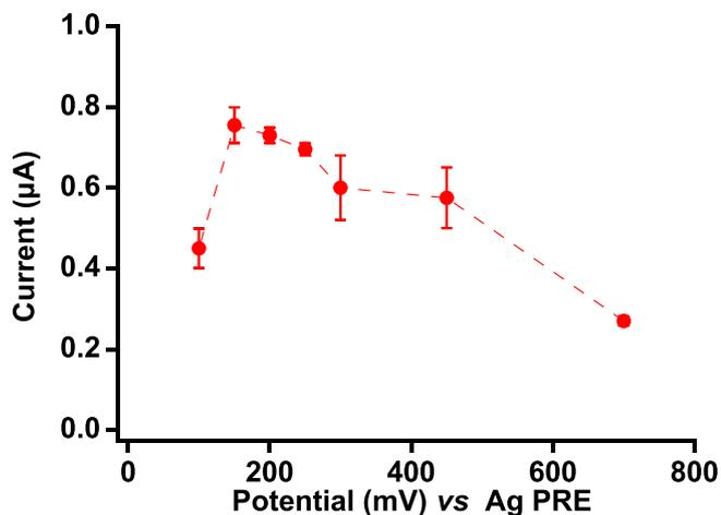
Fig. 4. Effect of applied potential on the amperometric response at  $\text{Au}_{\text{Nc}}\text{Pt}_{\text{Nf}}$  electrode towards the detection of 1 mM glucose.
