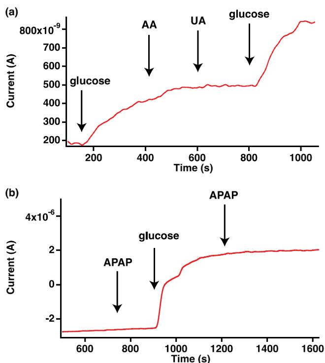
**Fig. 6.** Current-time response curve of the Au<sub>Nc</sub>Pt<sub>Nf</sub>/GOx biosensor to several interfering species in PBS 0.01 M pH 7.4 at +0.15 V (vs. Ag PRE). (a) 0.5 mM glucose, 0.1 M AA, 0.01 M UA and (b) 1 mM glucose, APAP 0.015 M and 0.045 M first and second injection, respectively.
