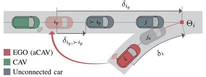
Fig. 2. EGO (vehicle  $i$ ) performing a merging maneuver by placing projection  $i_p$  right ahead another CAV, which can cooperate by reacting to it. The point before which the maneuver has to end is denoted  $\Theta_i$ .
