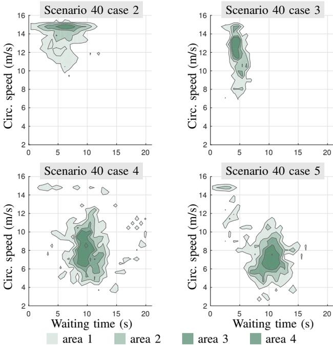
Fig. 7. Contour plots of waiting time-circulating speed 2D histograms for four selected cases (Table II). Every area  $i$  represents the subset  $\mathcal{S}_i$  (27) containing the samples whose probability of appearance is between  $p_i$  and  $p_{i+1}$ . With  $p_i$  being the  $i$ -element of vector  $\mathbf{p} = [0.1, 0.3, 0.5, 0.7, 0.99]$ .
