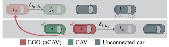
Fig. 4. Relevant vehicles to be taken into account by vehicle  $i \in \mathcal{A}^a$  when calculating speed references  $\bar{v}_i$  and  $\bar{v}_{i_p}$  to perform a lane change maneuver.
