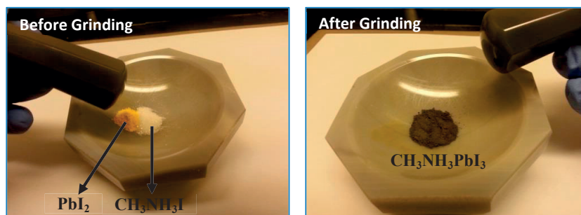
Figure 1.6 An experiment showing the low formation energy of MAPbI 3 from PbI 2 and MAI precursors. The solid state reaction between PbI 2 (yellow powder) and MAI (white powder) immediately takes place by gentle grinding of the two precursors at room temperature using a mortar and pestle for ~ 1-2 minutes resulting in MAPbI 3 perovskite (black grey powder in the right image). As mentioned in the text, the formation energy for MAPbI 3 from PbI 2 and MAI is ~ 0.1 eV (compare it, for example, with > few eV for BaTiO 3 perovskite synthesized from TiO 2 and BaCO 3 precursors, which needs a much higher reaction temperature (above 800 °C) for the solid state reaction to take place [61], [62]).
