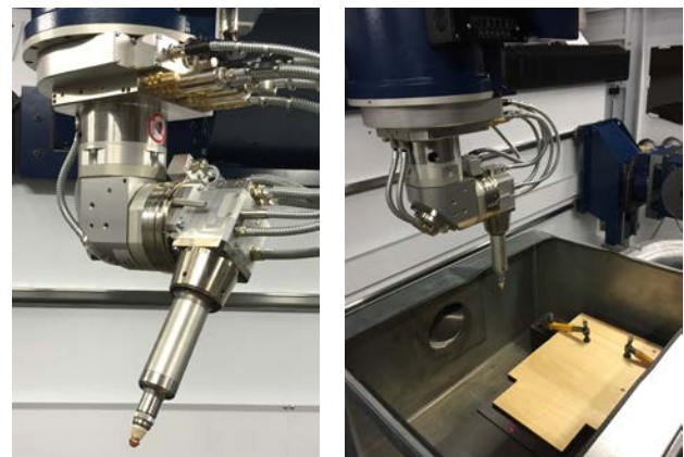
Figure 18: 5-axis 6kW CO2 laser system setup for LVL cutting
