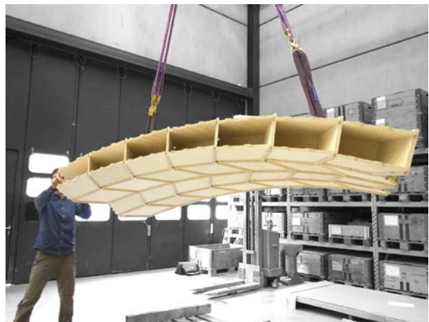
Figure 15: Double-layer Miura-Ori Folded Surface Structure made from LVL using closed-slot MTSJ, 2015 [8]
