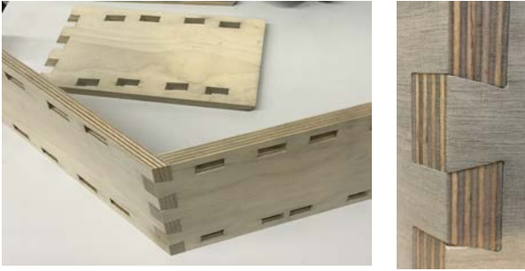
Figure 21: 15mm thick plates for a CSS [7] scale prototype, cut with a 5-axis equipped abrasive waterjet cutting system. Due to the cut width of only 0.6mm, no notches are needed.
