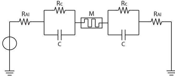
Fig. 3. Equivalent circuit for the simulation of the electrical behavior of a Memristive Biosensor by [11] extended here to include long electrical connection by Al lines.
