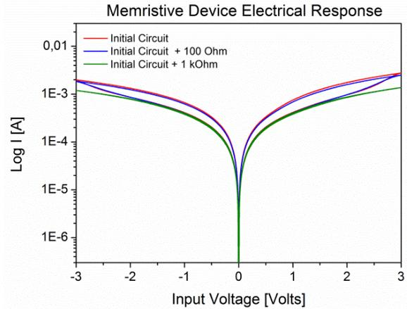
Fig. 4. Computationally obtained semi-logarithmic current to voltage results for the case of Memristive Device. The initial memristive curve becomes narrower for the addition of 100 $\Omega$  resistance in series to the Memristive Device and totally disappears for a total resistance of 1k $\Omega$ .
