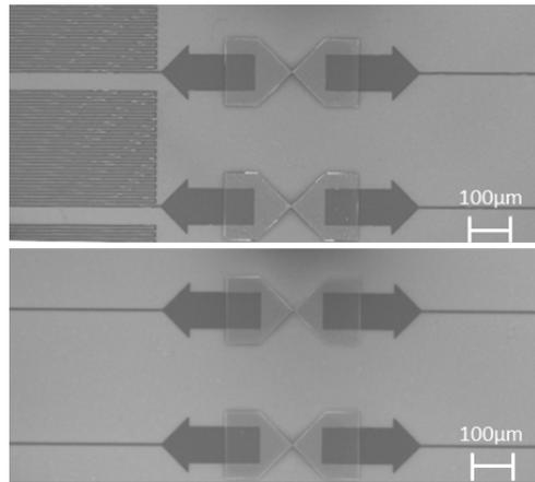
Fig. 2. Morphological SEM analysis of chips with two different configurations of Al metal lines: 10 k $\Omega$  (above) and 1 k $\Omega$  (bottom) in series to memristive nanowire devices.
