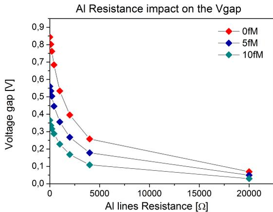
Fig. 5. Results by simulations concerning the impact of the resistance introduced by Al connections on the electrical response of the Memristive Biosensors with increasing concentration of antigen uptake: 0 fM (red); 5 fM (blue); 10 fM (green).
