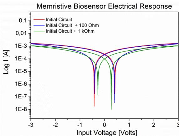
Fig. 6. Computationally obtained semi-logarithmic current to voltage results from the equivalent circuit (Fig.3). The initial memristive curve becomes narrower for the addition of a total resistance of 100Ω and 1kΩ with respect to the initial Memristive Biosensor equivalent circuit.
