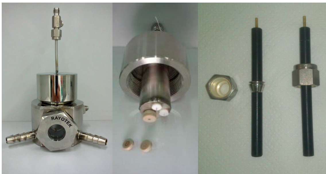
Figure 2.5. Reactor used for photoreduction experiments, the three-electrode cap and glassy carbon electrode equipped with high-pressure connection.
