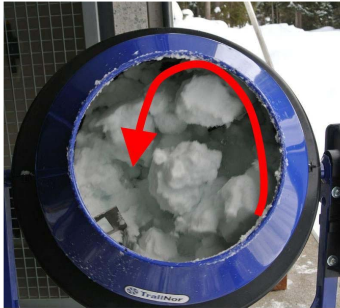
Figure 4.2: Granules in motion in rotating tumbler. One (of the two) mixing blades can be seen at lower left corner.
