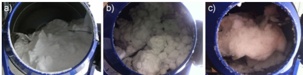
Figure 4.4: Snow inside tumbler for different experiments where (a) no persistent granules formed, (b) persistent-moist granules formed and (c) persistent-wet granules formed.
