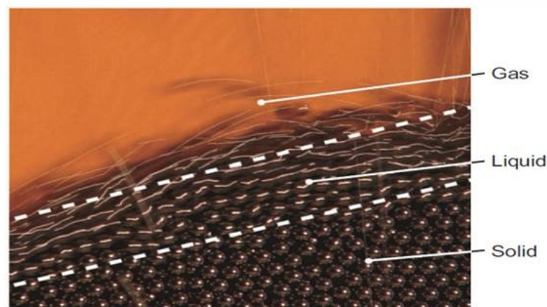
Figure 1.2: An illustration of the solid, liquid, and gas flow regimes obtained by pouring steel beads on a pile. From [ Forterre and Pouliquen , 2008].
