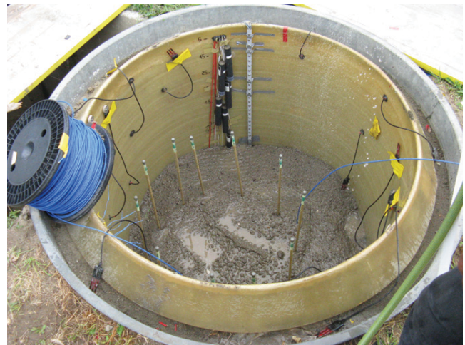
Fig. 4. Installation of the fiber optic cable. During uniform packing of the lysimeter, the soil is saturated and the fiber optic cable is wrapped around a bamboo-stick structure, which is removed after filling.
